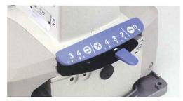
Stitch shape can easily be changed over between (3) and (3) button-hole configurations only by operating the lever. In addition, this single machine is able to sew two different kinds of buttons to save space and increase availability. (MB-1377)
