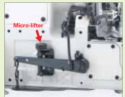
Bottom and top differential-feed micro adjustment mechanism
