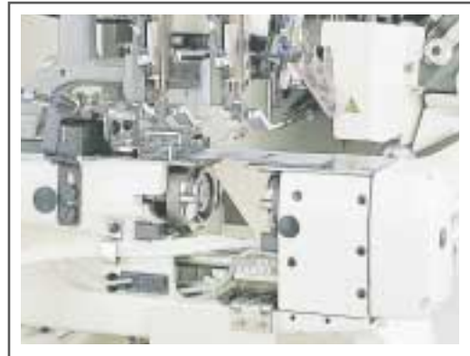
● With a maximized distance between hooks
